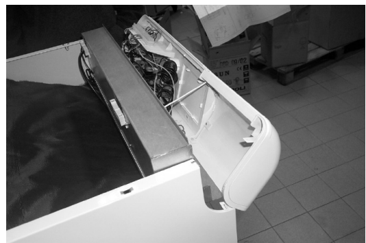
Fig. 6 - Turn the control panel forwards.
